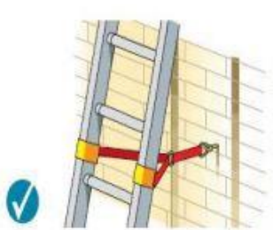
Tying near the base
